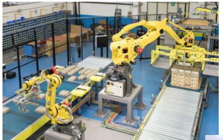
Robotic low-level palletizer with robotic pallet forming manipulator
